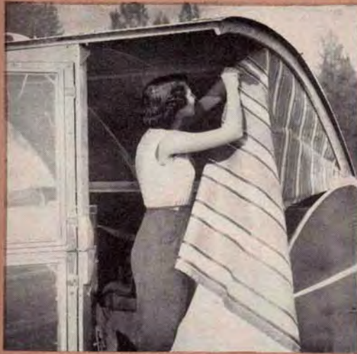
Fabric walls enclosing kitchen area are attached with grommets and turn buttons. Use heavy awning cloth
